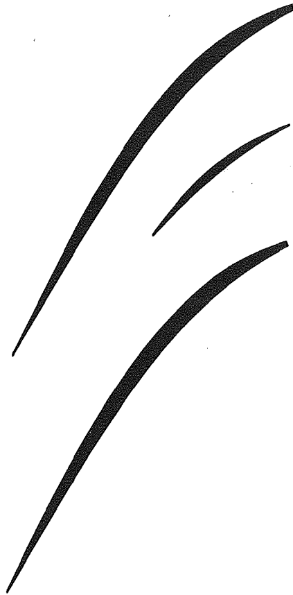
Fig. 3 Rotor cascade with splitter vanes
